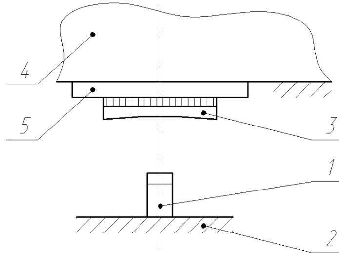
Fig. 1 – Scheme of a bench for burnisher face photographing where 1 – object under study; 2 – white screen; 3 – lens of digital photo camera; 4 – digital photo camera; 5 – round flash
