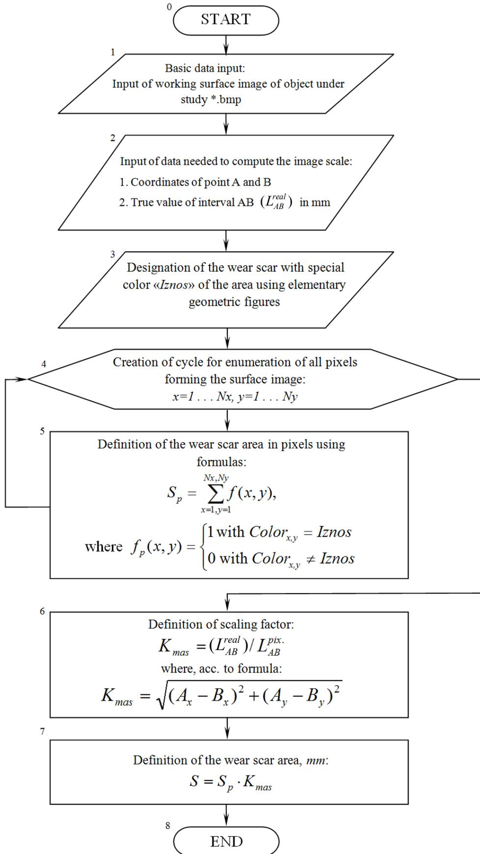
Fig. 2 – Flow chart of surface wear area determination algorithm
