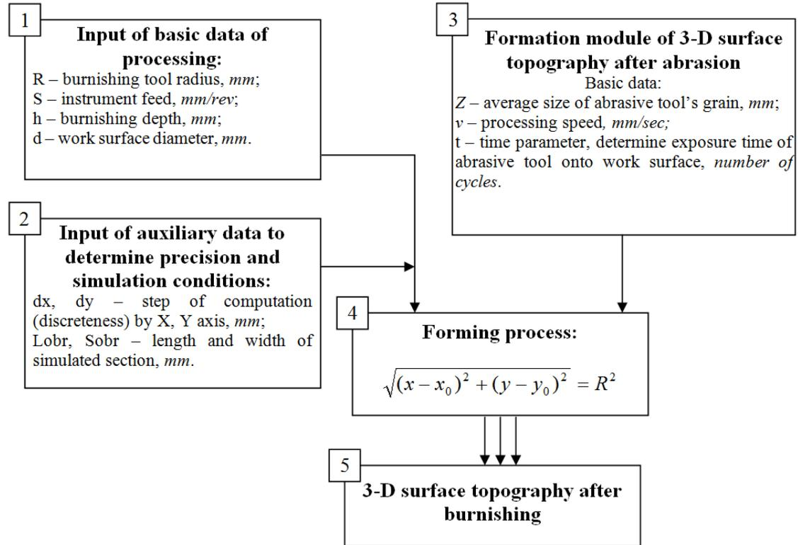
Fig. 3 - Burnishing process block schematic diagram
