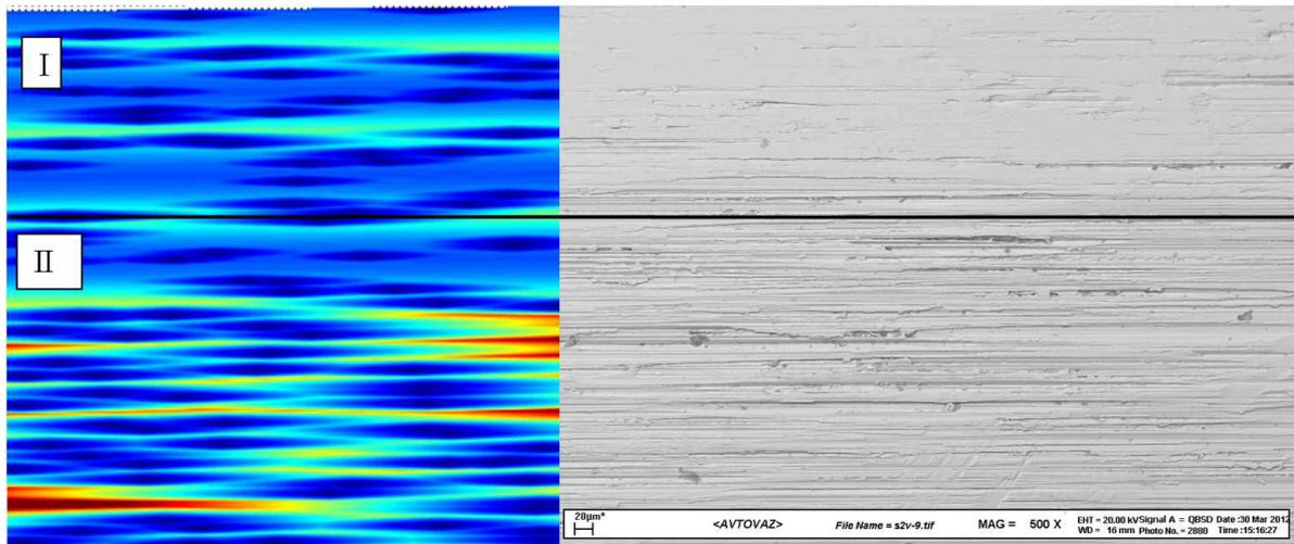
Fig. 5 – Contention of surfaces (plane view), achieved from electron microscope (right) and computer-simulated (left). Roman figure I – burnished surface patch, II – grounded surface patch
